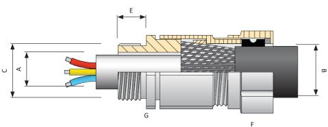
Designed to the B.S. 6121 standard, the IGCX is a robust metallic range of cable glands for industrial applications which provides an outer seal and armour clamping, grounding and earthing.
